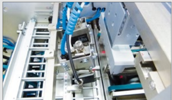
Glue application in the XP-250.1 knife folding unit with optional glue inspection
