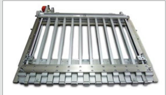
Improved setup times by using combi plates with sheet stop/deflector combination
