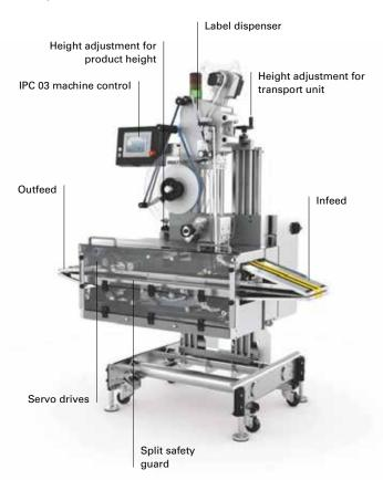
Sealing labels on a backing strip width of 15, 20 or 25 mm are dispensed onto the rear edge of the product and then applied around it by means of a top air blowing nozzle and a presson unit. Servo drives ensure the maximum output and precision are achieved. Thanks to exchangeable dispensing edges and format plates with defined pitch and sensor positions, the L 350 can be converted quickly and conveniently to other label widths or paper formats.
