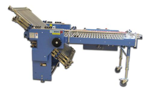
The Digi-FW 780/6 is a modification of the 8-page folding unit used in the B 30S Perfection folding machine. This unit can communicate with other digital machines and can run high speed production. Its MBO engineering makes it one of the fastest and most durable folding machines available. Because the Digi-FW 780/6 can be controlled independently it can be used with a variety of older machines or machines from other suppliers.
