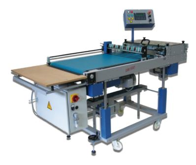
The SAB 550 is a shingled stream delivery specifically designed for processing multi-up production. Its adjustable flat belt infeed fills the width of the machine, ensuring a smooth and efficient sheet transfer for a variety of job formats, regardless of how many products are coming through. Thanks to MBO's Modular Advantage, the SAB 550 Shingled Stream Delivery is compatible with a wide range of finishing modules from MBO and Herzog+Heymann.
