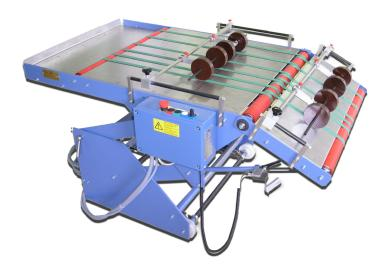
The 702 is a variation of the 701 delivery system. This machine utilizes the same batching process as the 701, allowing for highly efficient batch deliveries. The 702 is different from the 701 in that it has a pivoting infeed where the 701 is stationary. This makes the 702 more adaptable to machine height variances and it is also more ergonomic for operators.
