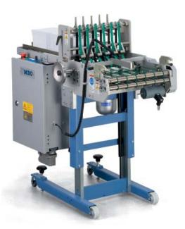
The KAS 30ME is a vertical delivery specifically designed for small format products. The infeed on this machine is a top and bottom spaghetti belt system which allows for greater control during spreading. Product remains under control because of a pair of stabilizing delivery guides on the tray. Additionally, the KAS 30ME is equipped with an independent self-control, meaning it can be used in a wider range of configurations including lines with older machines or machines from other suppliers.
