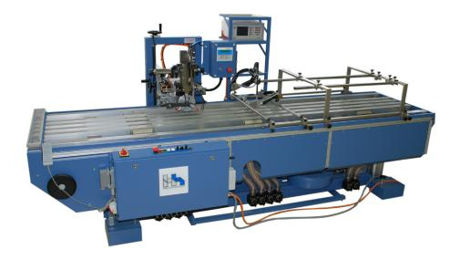
The 091.1 mailing table is very efficient way to fit multiple processes in a small amount of space. This machine can be mounted with a variety of components and each table can do one process every meter. Product is carried from one process to the next by the vacuum belt system. The vacuum system on this machine can detect the number of sheets on the belt and compensate by increasing or decreasing the suction strength.
