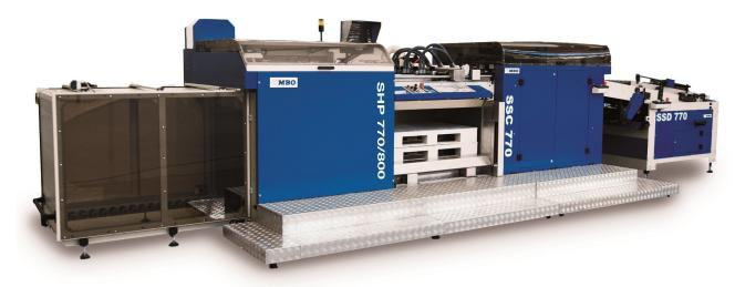
The SHP 800 is a high speed, high-pile stacker capable of matching production rates of the fastest modern presses. Without interrupting production, the SHP 800 System will automatically change pallets when triggered by a pre-programmed batch count or by reading codes from the web. Additionally, the SHP 800 streamlines the production process by automatically ejecting white waste and job changeover sheets - making it ideal for both inline or near-line configurations.
