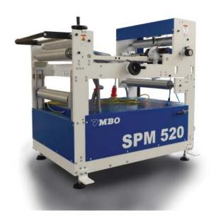
The SPM 520 is a specialty machine designed to handle split and merge tasks quickly and efficiently. This machine is set up in-line and will split and then re-align sheets at high speeds prior to entering the next stage of production. The basic model comes with a longitudinal knife to trim away any unwanted edges and there is an upgrade available to incorporate a gutter cut blade for center cuts.
