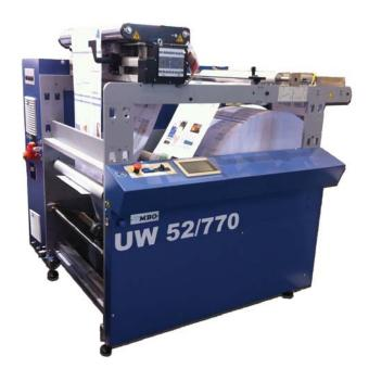
The UW 770 is a digital unwinding machine featuring dancer-controlled web tension and a center driven servo motor. It comes equipped with an electric paper lift, an integrated splice table, as well as a de-curling device making it easy to operate and quick to set-up. This machine is designed to be integrated into any digital printing or web finishing line.
