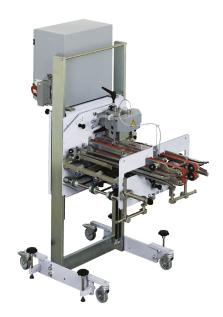
The Z2 is a knife folding unit from MBO that features a pivoting knife section which can be configured to perform an upward or downward fold. After the fold takes place, product can be delivered to either the left or right depending upon the operator's settings. The Z2 also features an independent self control, meaning it can be used in a wider range of configurations including lines with older machines or machines from other suppliers.
