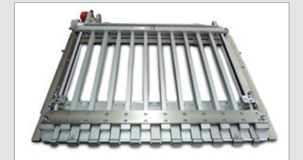
Improved setup times by using combi plates with sheet stop/deflector combination
