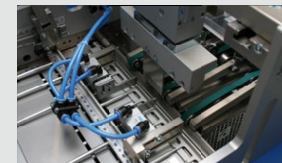
Strong and stable double-sided product alignment for best folding quality
