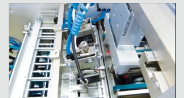
Glue application in the XP-250.1 knife folding unit with optional glue inspection
