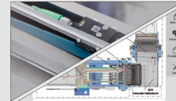
Optional sheet monitoring by photocells with touch screen control for a safe run
