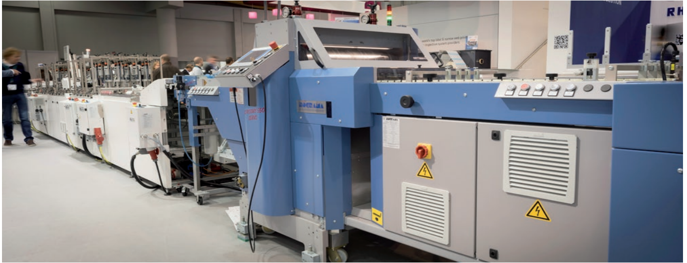
Packaging-Line „Stamina“, consisting of BSR 550 Servo with pallet feeder and Herzog + Heymann folding carton line.
