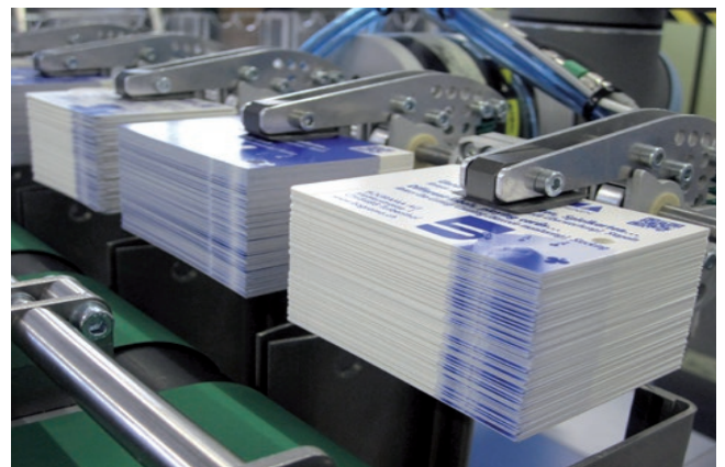
BSR 550 Servo in combination with „RoboStack“; Automated sorting and packaging solution for filling trays, banding or placing on a belt.
