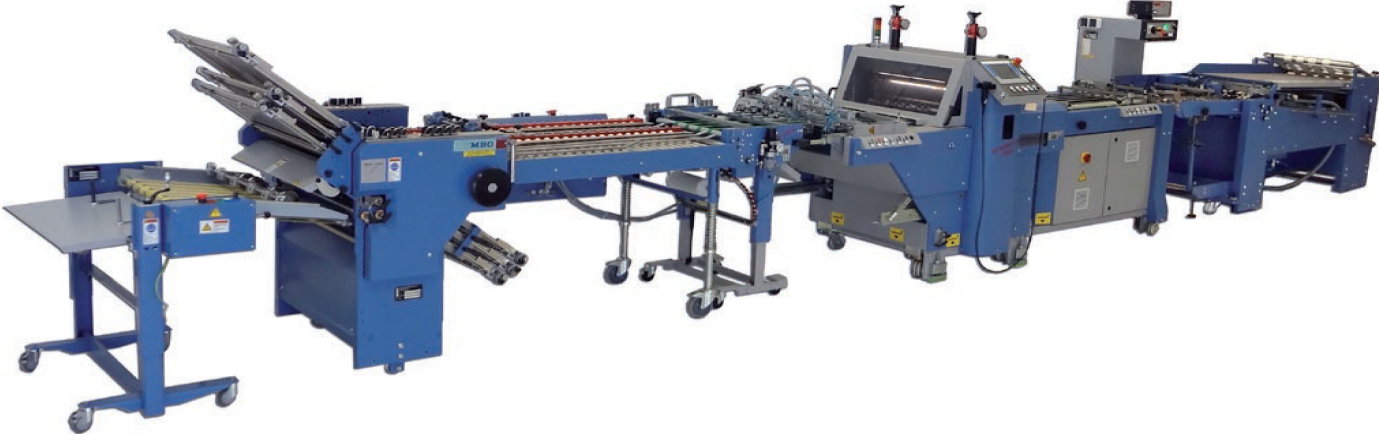
Production line consisting of upstream continuous feeder, BSR 550 Servo, UEB 550 B and downstream buckle plate folder.
