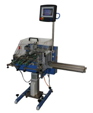
The XS 300 is a knife folding unit that has many MBO features. The knife on this machine features a kicker for batching and a back stop which adjusts location in order to reduce cycle times. After the knife fold process, paper can be fed out to the left or right side in order to suit a wide range of configurations. The XS 300 also comes with a vertical delivery cassette and a belt transfer cassette which are interchangeable depending upon the unit's position within a production line.
