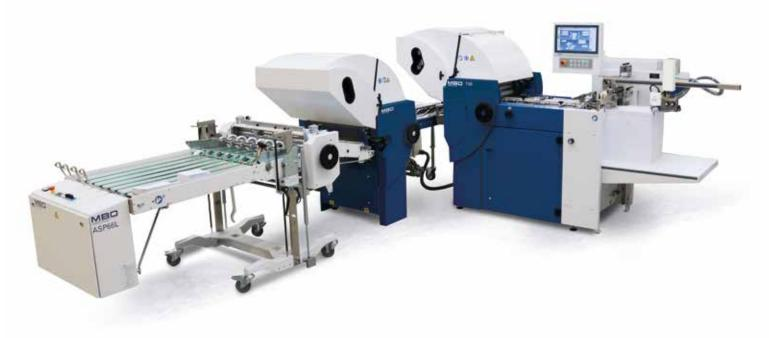
Automated T50 with pile feeder, folding unit II and ASP66L delivery.
