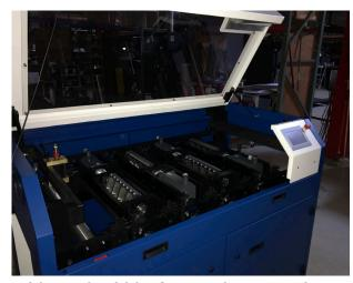
With a web width of 22" and an operating speed of up to 500 feet per minute, MBO's Dynamic Perforator can apply scalable cross and linear perforations to any digital web application.
