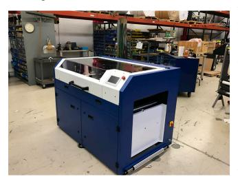
MBO's dynamic perforation solution is capable of parallel and perpendicular perforation at variable locations.
