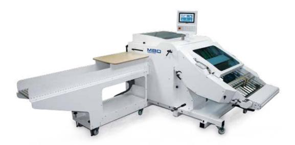
The A80 is the ideal delivery for the production of signatures. In the A80, the sheets first run through a pair of press rollers and are then transported to the collection shaft in single sheet or shingle stream mode. The integrated jogger device creates precise product stacks. These are then supplied ready for removal in perfect quality and at a convenient height.
