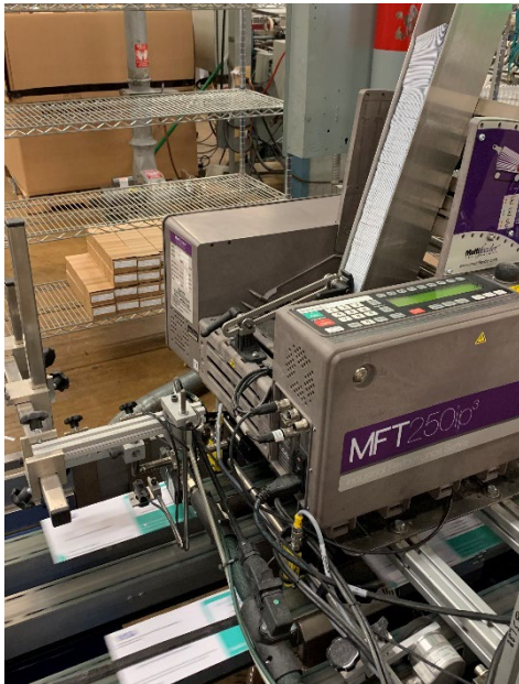
After the forms are trimmed and folded, embossed cards are affixed and scanned for an accurate match on the MBO Folding Systems
