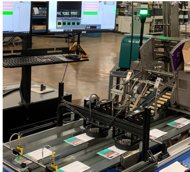
After the forms are trimmed and folded, embossed cards are affixed and scanned for an accurate match on the MBO Folding Systems
