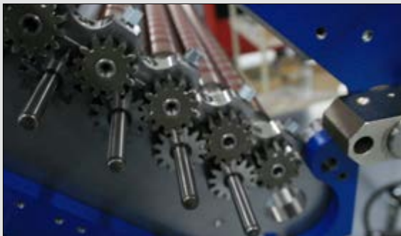
Tried and tested, low-maintenance gear drive
