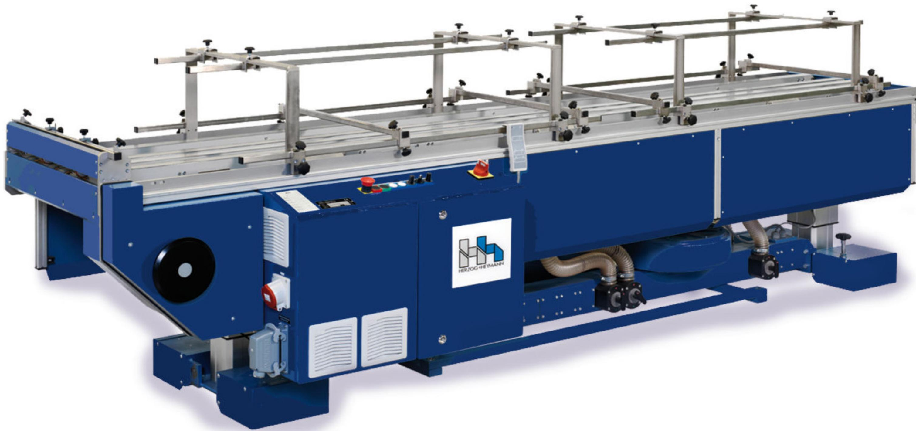
The 091.1 mailing table is a very efficient way to fit multiple processes in a small amount of space. This machine can be mounted with a variety of components and each table can do one process every meter. Product is carried from one process to the next by the vacuum belt system. The vacuum system on this machine can detect the number of sheets on the belt and compensate by increasing or decreasing the suction strength.
