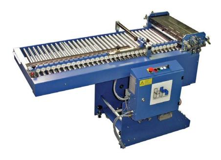
The 281 cutting unit from Herzog+Heymann is a very adaptable cutting machine. This machine can do many cutting functions, all that is needed is the appropriate knife. Because of its versatility there are a number of options available to the 281 that allow one to make the 281 cutting unit even more useful.
