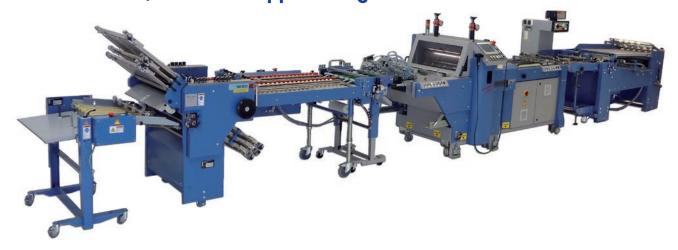
Production line consisting of upstream continuous feeder, BSR 550 Servo, UEB 550 B and downstream buckle plate folder.
