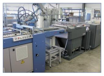
BSR 550 Servo with Tecnau unwinder/cross cutter
