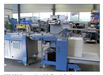
BSR 550 Servo with mobile flat pile feeder
