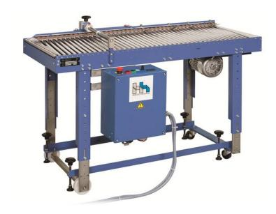
The 407 is a cross carrier table used primarily for product alignment during transfers between modules. The high-speed guide allows for superior alignment accuracy as product moves along the table. This machine is independently driven and has an independent self-control. Because of the independent self-control, the 407 Cross Carrier can be configured to work with a wide variety of modern machines, older machines, or machines from other suppliers.
