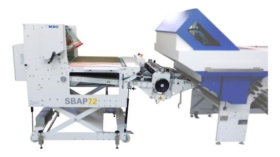
The SBAP Series is a line of high-performance vertical stacking delivery systems for signature production. Because the signatures are stacked vertically, this machine has a considerably larger holding capacity than most stream deliveries. All SBAP deliveries come equipped with a pressing station, an integrated marking device, and an independent self-control feature - making them highly compatible across MBO finishing modules in both offset and digital print environments.
