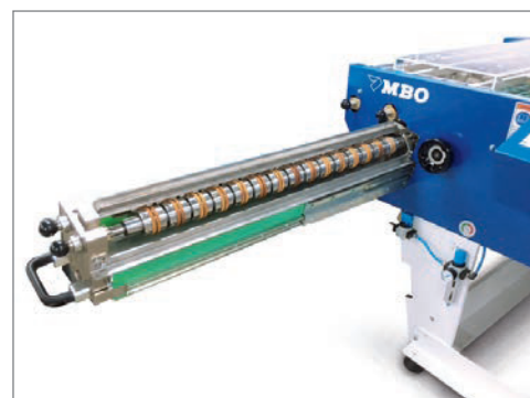
Slitter shaft cassette
