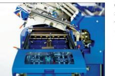
Swinging up of crossfold knife area and sliding out of threefold knife area: For free accessibility to the foldrollers and slitter shafts, for adjusting, cleaning and removing of paper.
