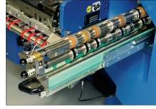
The slitter shaft cassette included as standard equipment reduces changeover times. In an ergonomically favourable height the cassette can be easily and quickly drawn out on the operator side, allowing the precise adjustment and positioning of the knives. Moreover, all needed strippers (like e.g. edge trimming or gully cut device) can be mounted directly on the cassette outside the machine.
