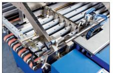
The sheet stop in the crossfold can be used as a waste paper ejector. Double or heavily misfolded sheets are ejected during production without interruption of the production flow. Immediately after the ejection the waste paper ejector closes again and the production is continued without any disturbance. Novel track-keeping tooth belts ensure optimal transportation of sheets.
