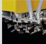
VACULIFT III VACULIFT III ensures a constantly optimal sheet separation due to the motor-driven
