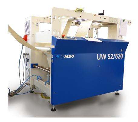
The UW 520 is a digital unwinding machine featuring dancer-controlled web tension and a center driven servo motor. It comes equipped with an electric paper lift, an integrated splice table, as well as a de-curling device making it easy to operate and quick to set-up. This machine is designed to be integrated into any digital printing or web finishing line.
