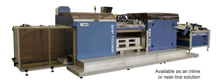
The High-Pile Stacking Solution from MBO America is a fully-automatic cut sheet palletizing production system that gives printers the ability to create palletized stacks from a 30 inch web. Because the system can produce up to a 28" x 40" sheet, commercial printers can integrate digital and inkjet web applications into a traditional commercial finishing workflow. With the High-Pile Stacking Solution, a hybrid printer can minimize the production workflow bottleneck at
