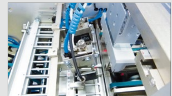
4 Glue application in the XP-250.1 knife folding unit with optional glue inspection
