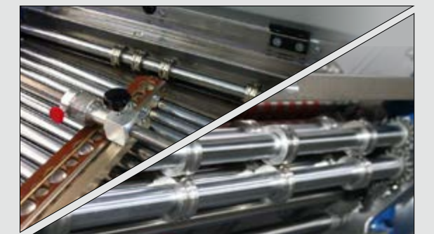
Pre- and rear slitter shaft for cutting, scoring and perforating
