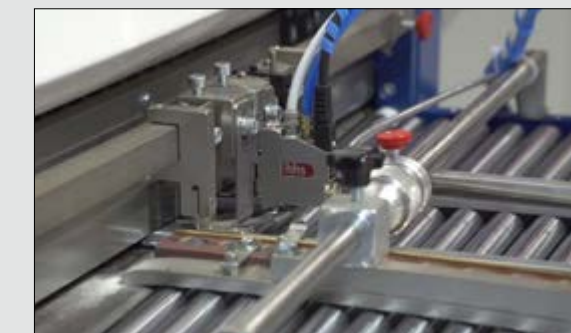
Integrated gluing system for fold gluing
