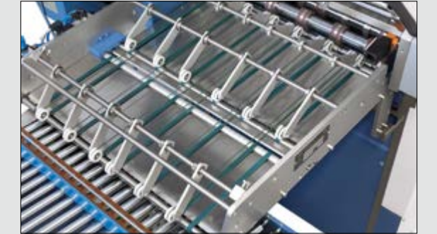
Transfer unit with sheet ejector unit
