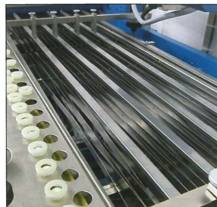
Belt register table with side-lay for the alignment of low paper grammages.
