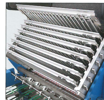
② 1st folding unit KL 112.1 with 16 folding pockets. The folding pockets are located in position.
