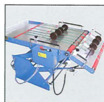
Flat track delivery type 702 with movable infeed for ergonomic working.
