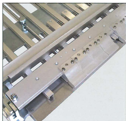
Segmented upper pocket mouth for hotmelt gluing in the folding machine.
