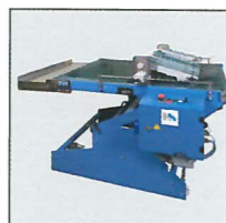
Flat track delivery type 703 with flat belt for products with small formats.
