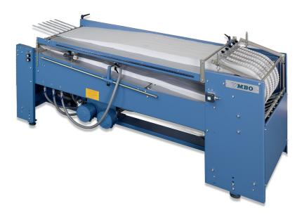
The R Series continuous feeders were designed to increase the production efficiency of high volume jobs. Paper is loaded along the top conveyor and then looped around to the bottom conveyor, doubling your load capacity and creating a horizontal queue of paper which can be fed through at high speeds. Because of its innovative design an operator can continually load paper onto the top conveyor without ever stopping production.
