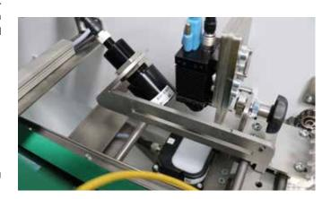
The cameras in the MBO VT50 measure the position of the cutting marks relative to the outer edge of the paper.
