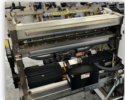
Cutting cylinder cassette shown in open position for access.
