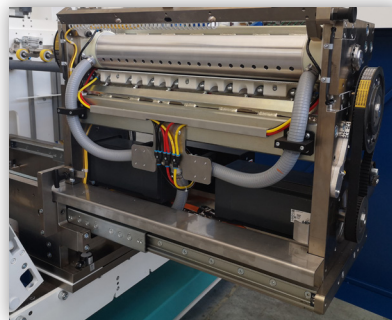
Cutting cylinder cassette shown in open position for access.
