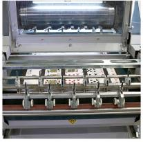
Break out elements for deflecting the sectiontion grids and delivering the products. Short setup times, toolless adjusting
