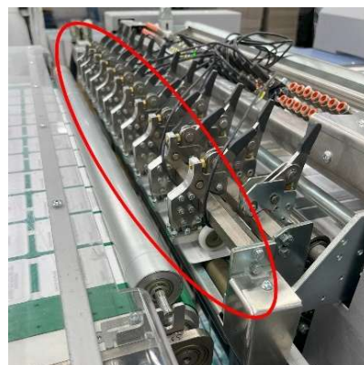
9) Automated stripping, short set-up, toolless adjusting. Blind card ejection. Sensors for card counting.
