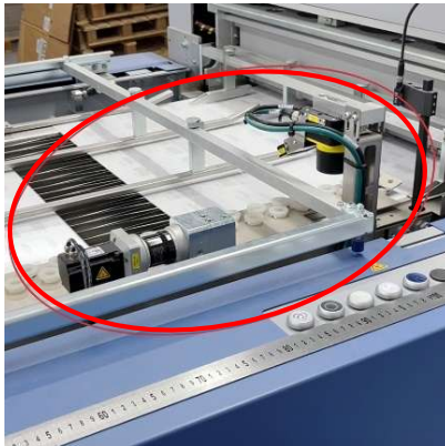
6) Dynamic side alignment. Print mark recognition with camera system
