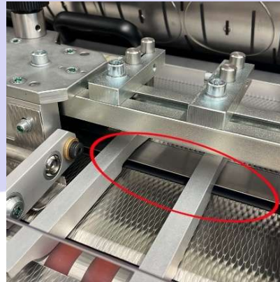
5) Ultrasonic double sheet inspection with automatic ejection for non-stop operation
