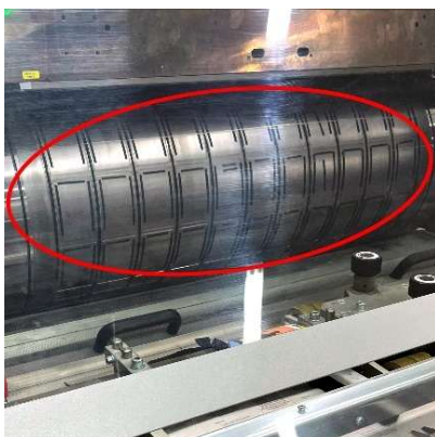
8) Flexible die-cutting technology for rounded corners round products, inner die-cuts. Changeover in 10 min.
