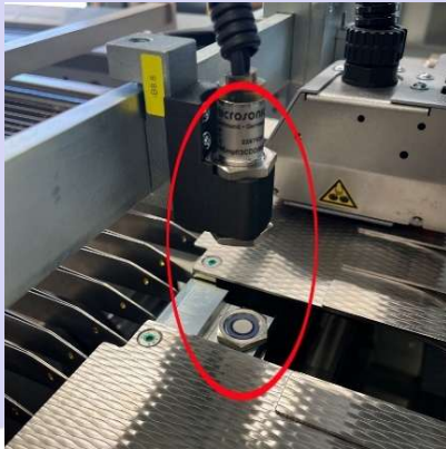
5) Ultrasonic double sheet inspection with automatic ejection for non-stop operation
